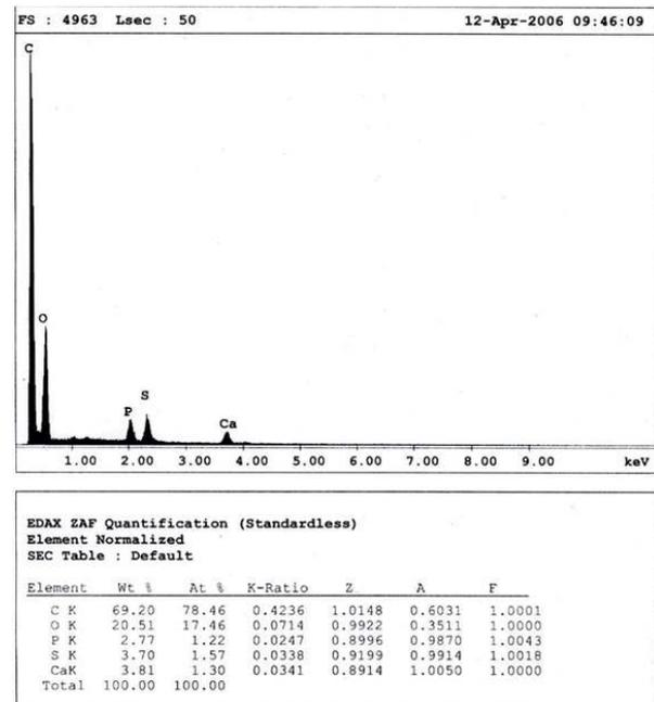
**Figure 1.** Typical printout for X-ray Microanalysis showing Chemical Elements at their KeV peak; Note the chart with wt % recorded. Specimen not coated with gold
