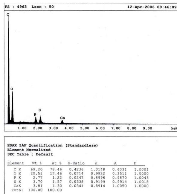
**Figure 1.** Typical printout for X-ray Microanalysis showing Chemical Elements at their KeV peak; Note the chart with wt % recorded. Specimen not coated with gold
